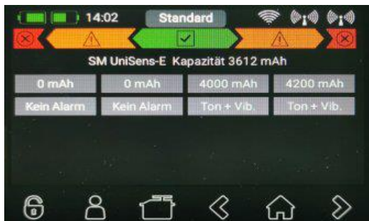
Alarms are defined directly in this widget in the transmitter.
